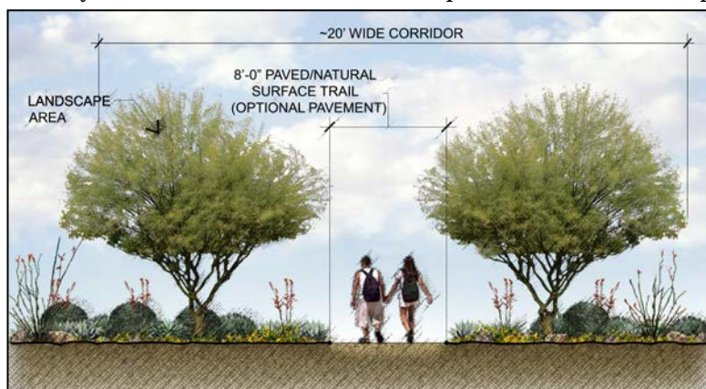
Figure 24: Local Area Trail Typical Cross-Section Detail
