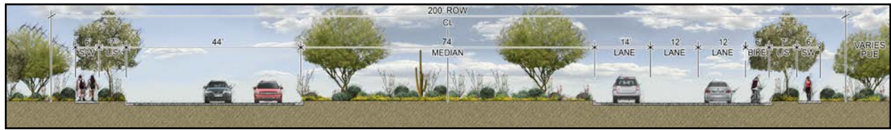
Figure 28: 6-Lane Parkway Cross Section
