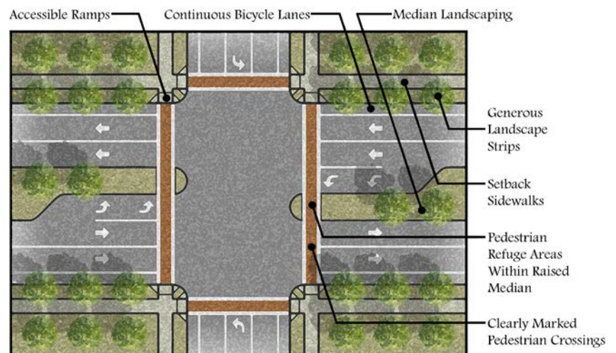
Figure 27: Typical Intersection Design 4-Lane Major Street and 2-Lane Collector Street
